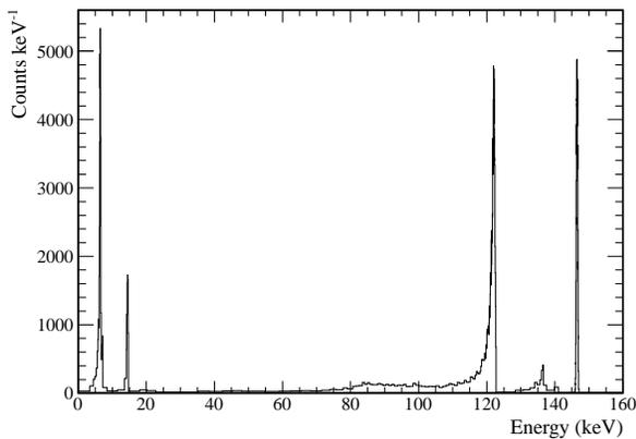
Figure 1. A typical spectrum of one CdZnTe pixel obtained with a  $^{57}\text{Co}$  radioactive source, which emits strong  $\gamma$ -ray lines of 6.40, 7.06, 14.4, 122 and 136 keV. The 146 keV peak is produced by the on-chip test pulsar. Events that only the center pixel is triggered are collected. Data were taken at 278 K temperature and -450 V high voltage for one day.
