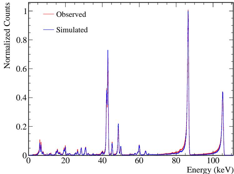
Figure 10. Comparison of the simulated  $^{155}\text{Eu}$  spectrum with the observed one. The detector is operated at 278 K temperature and -450 V high voltage. All of pixels are used except for edge, corner, and dead pixels. Single-pixel events in which a trigger of the center pixel is solely activated are collected. The observed energy resolution in FWHM is 0.8 keV at 86.5 keV. Both spectra are scaled by the 86.5 keV peak counts.
