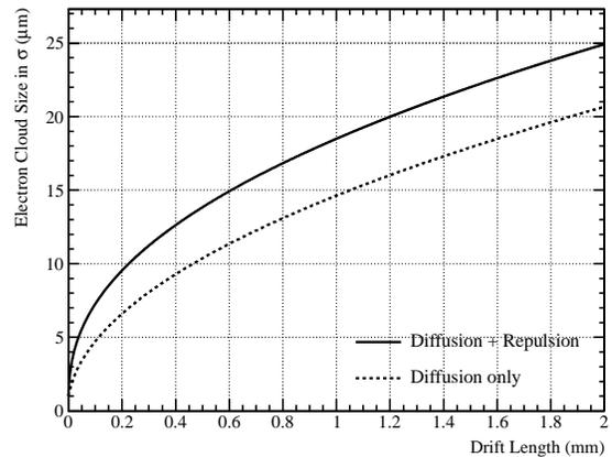
Figure 4. Standard deviation of electron cloud size at a 60 keV energy deposition with an initial radius = 1  $\mu\text{m}$ . The solid and dotted lines represent electron cloud size with and without electrostatic repulsion, respectively. The applied high voltage is 450 V and temperature is 5 degree. Although the electron mobility is set to be  $10^{-3} \text{ cm}^2 \text{ s}^{-1} \text{ V}^{-1}$ , the curves are nearly independent of it.
