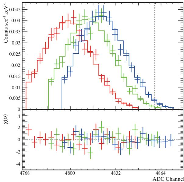
Figure 5. 59.5 keV line spectra taken with  $^{241}\text{Am}$  at different 3 high voltages of 300 (red), 400 (green), and 500 V (blue). The vertical dotted line represents the expected peak with no electron trapping [ $\text{Ch}_0$  in equation (3)]. The lower panel shows the fit residuals in term of  $\sigma$ .
