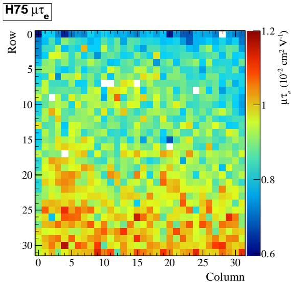
Figure 7. Map showing obtained electron mobility-lifetime products for the 32×32 pixel array in a CdZnTe hybrid.
